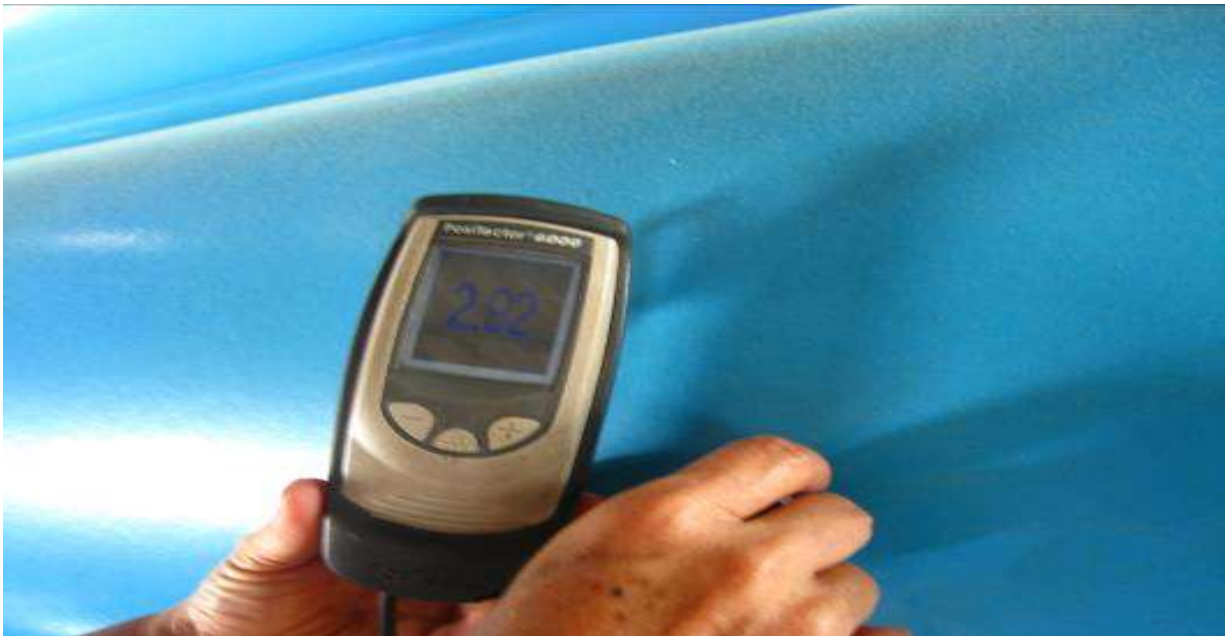
103.6.16 24" 管-膜厚量測 2.92mm > 2.5mm
