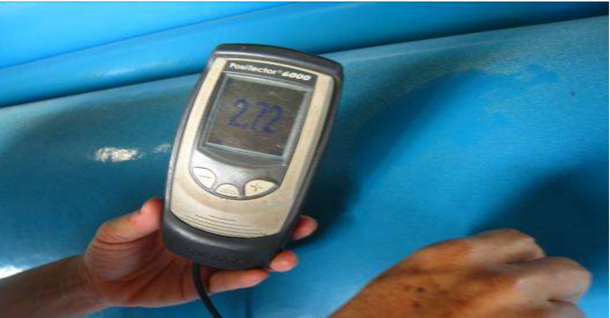
103.6.16 24" 管-膜厚度量測 2.72mm > 2.5mm
